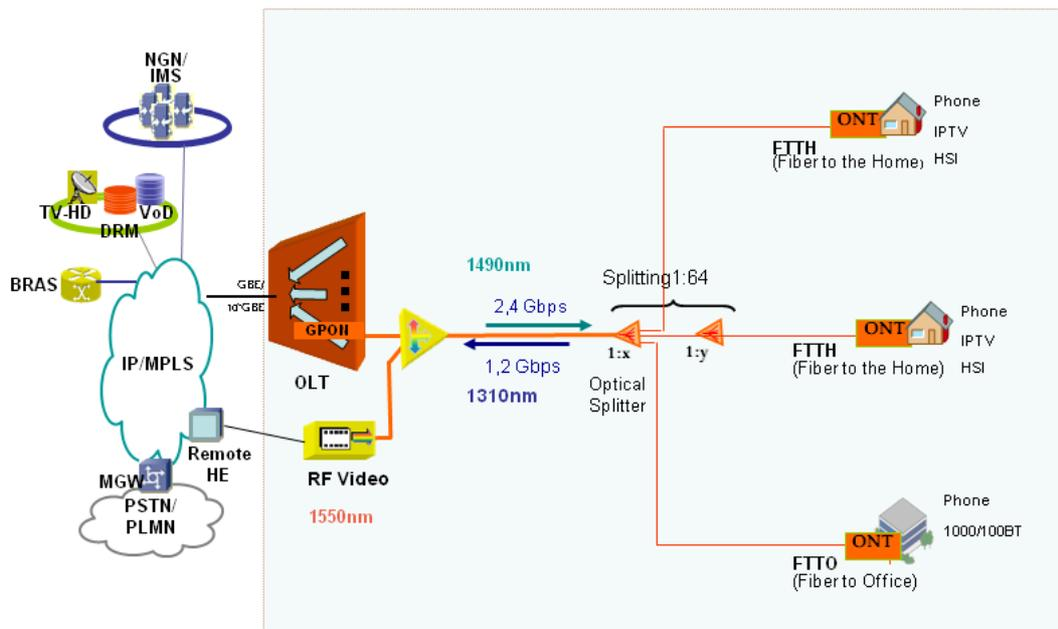
Figure 7: Current GPON deployment
