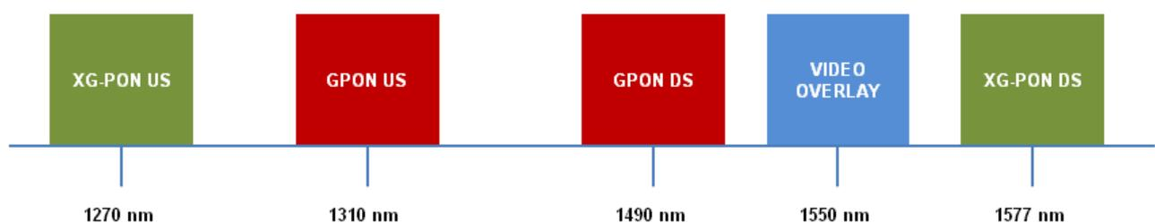
Figure 3: ITU-T G.987 wavelength plan
