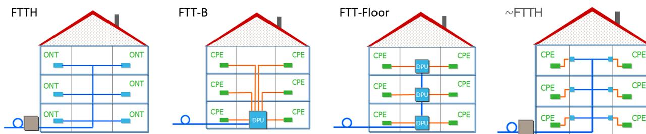
Figure 2: FTTB variants differ in where the fibre terminates.
